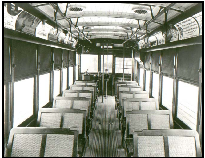
Trolley car seats were constructed to flip forward and back depending on the direction of travel.
