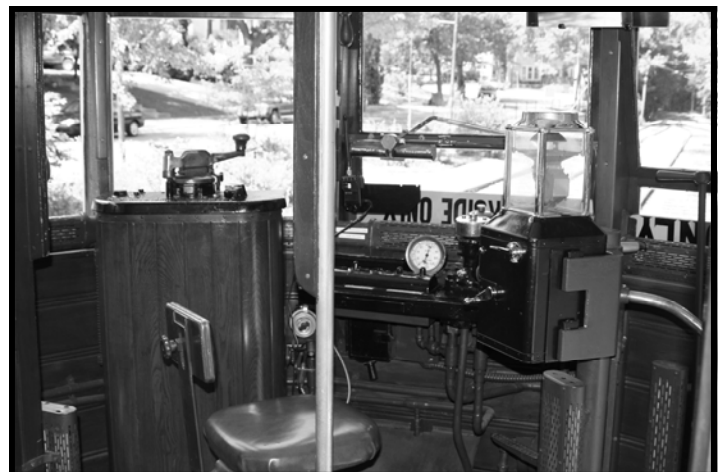
Typical motorman controls at the head end of the trolley car.
